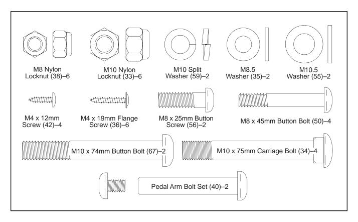
Identify the Front Stabilizer (10). While another person lifts the front of the Frame (1), attach the Front Stabilizer to the Frame with two M10 x 75mm Carriage Bolts (34) and two M10 Nylon Locknuts (33). Make sure that the Front Stabilizer is turned so the Wheels (22) are not touching the floor.
